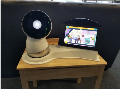
Figure 3: An integrated social robot platform that supports different game “tasks”.
